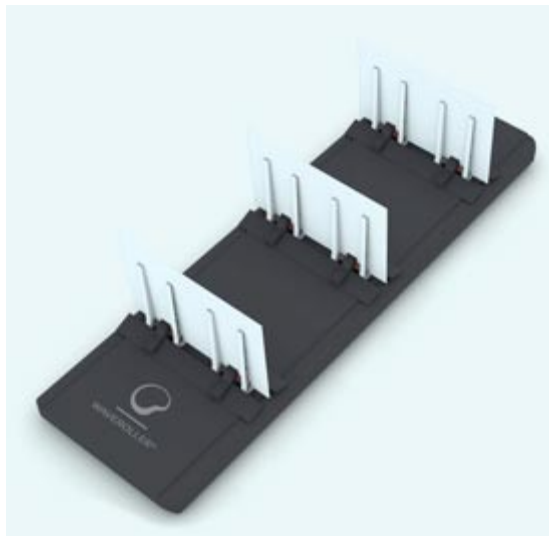
Figure 11: Graphical illustration of WaveRoller 3x100kW prototype.
